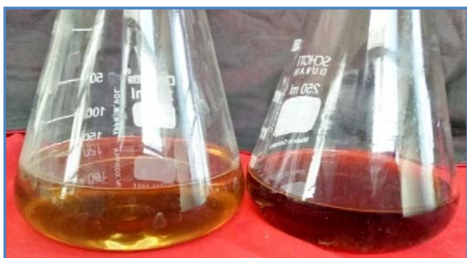
Plate 1: Plant extracts, (A) before addition of \text{AgNO}_3 (B): after formation of silver nanoparticles
