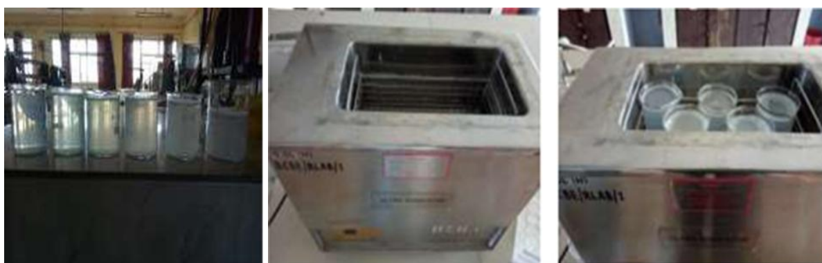
Plate 1: Dissolving Nanoparticles in distilled water and kept in Ultra Sonicator
