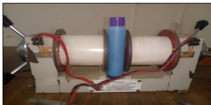
Fig 2: Seeds placed in a rectangular shaped bottle with water in the space between the two bars of the electromagnet
