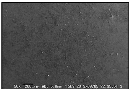
Fig 2b: SEM images of non-polished surfaces of NiA1
