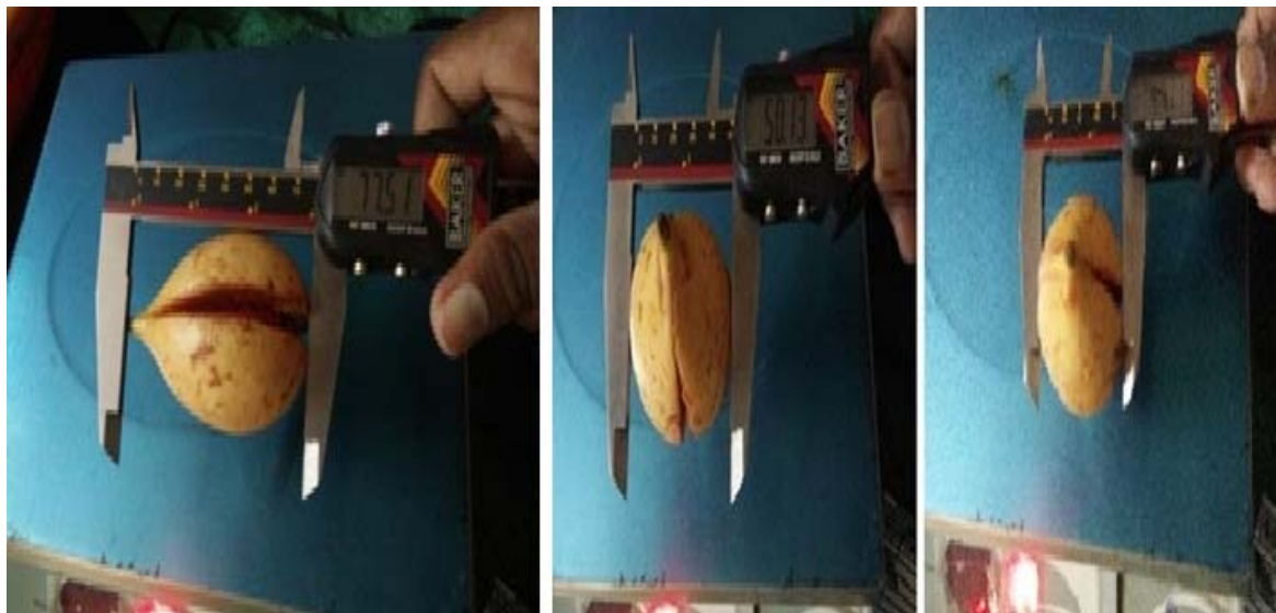
Plate 1: Measurement of length, breadth and thickness of fruit with the help of Vernier caliper.
