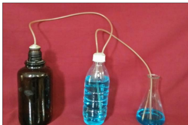
Fig 2: Empirical Model of Pneumatic Solution Dispenser for automatic application of nutrient solution to plant
