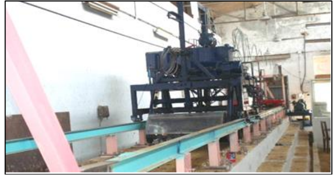
Fig 1: Experimental soil bin
