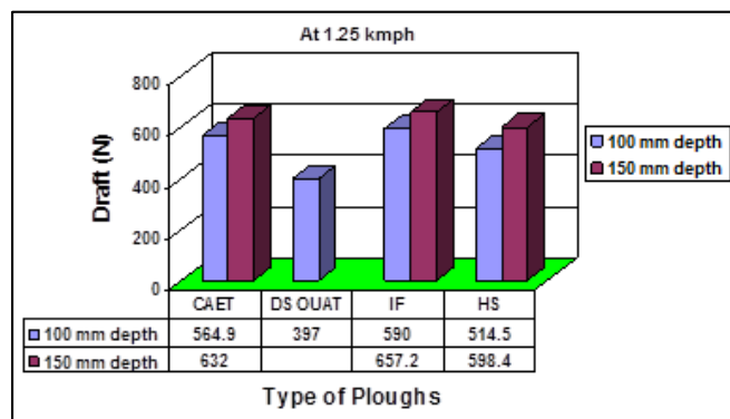
Fig 4: Drafts of test ploughs at 100 mm and 150 mm depth at a speed of 1.25 kmph.
