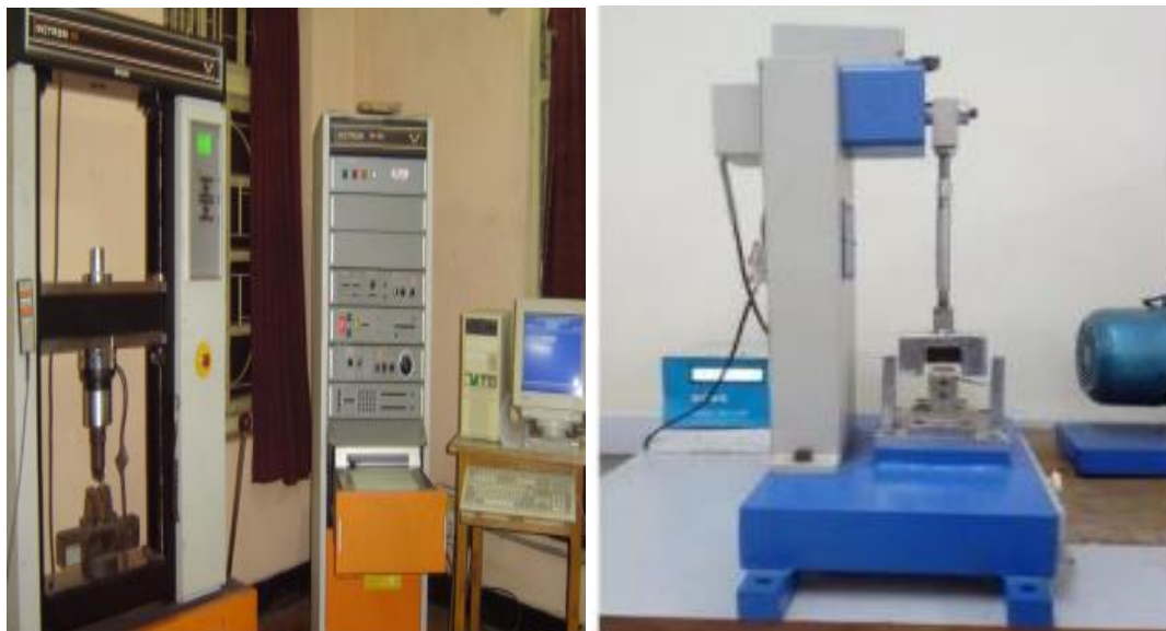
Universal testing machine for Tensile and Flexural Strength
