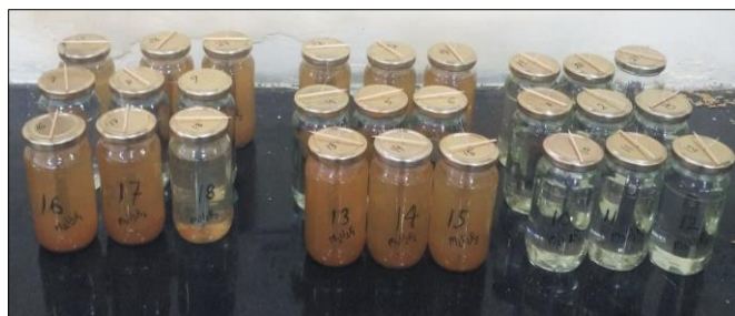
Fig 4: Corrosive effect of UAN: Water on different metals after 24 hrs
