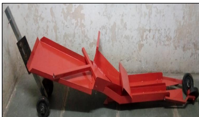
Fig 5: Developed paperpot transplanter
