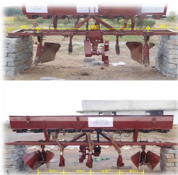
Fig 5: Back view of modified broad bed furrow machine
