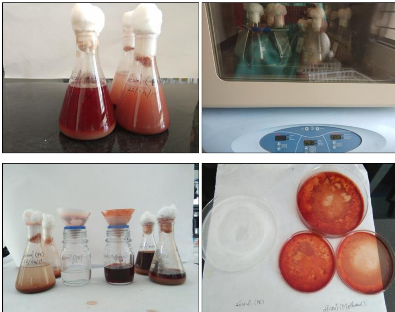
Fig 1: Extraction of A. catechu in methanol and water
