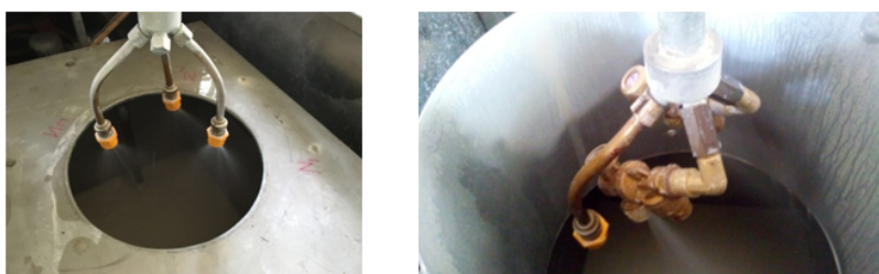
b. Discharge through CCO plates during test
