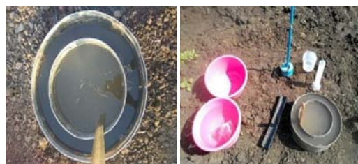
Fig 1: Double ring infiltrometer
