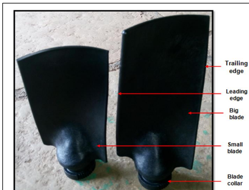
Plate 1: Blades used in blower
