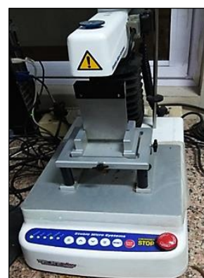
(A) Probe: Warner-bratzler blade with rectangular hole
