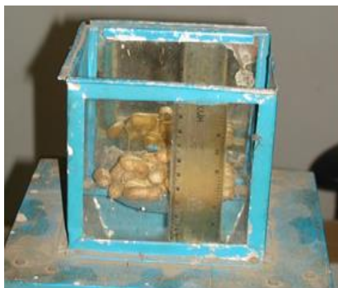
Fig 5: Determination of angle of repose
