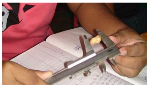
Fig 1: Measurement of length, width and thickness of groundnut
