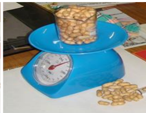
Fig 3: Measurement of bulk density
