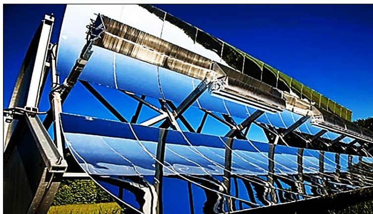
Fig 1: Parabolic trough collectors
