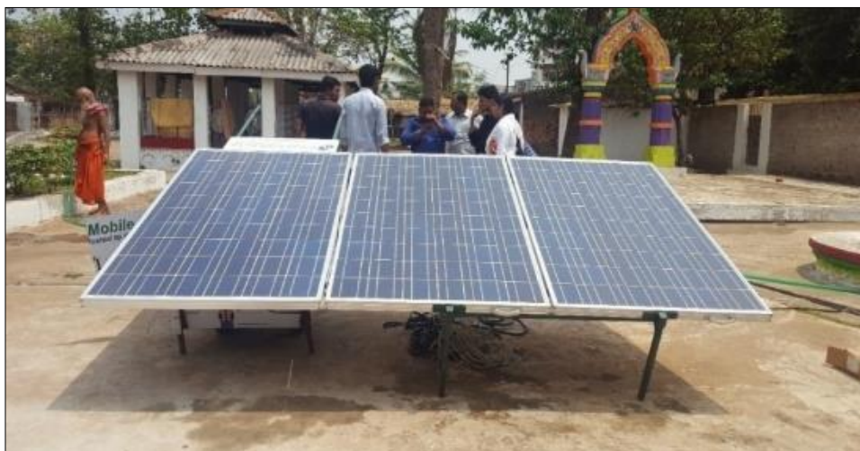
Fig 4: Display of folding type solar panel over a flatbed stand
