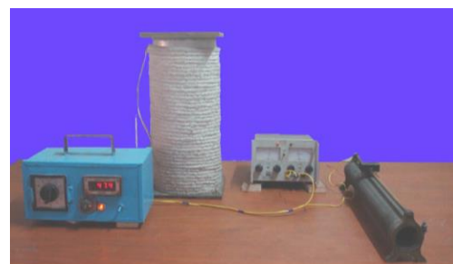
Fig 1: Thermal conductivity apparatus (adapted from Jeevarathinam and Pandiarajan, 2016)
