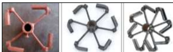
Fig 7: Developed metering device of 4, 6 and 8 number of cups
