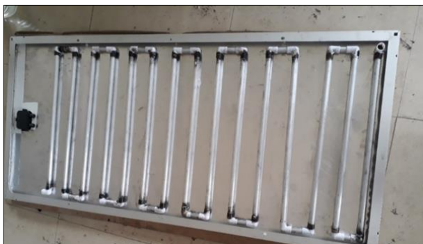
Fixing of aluminium air flow channel at back side of the PV panel
